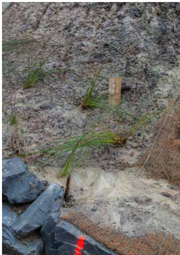
The rock toe in August 2019 showing sediment runoff from Plot 9 (control/no product) being trapped on the rock toe.
