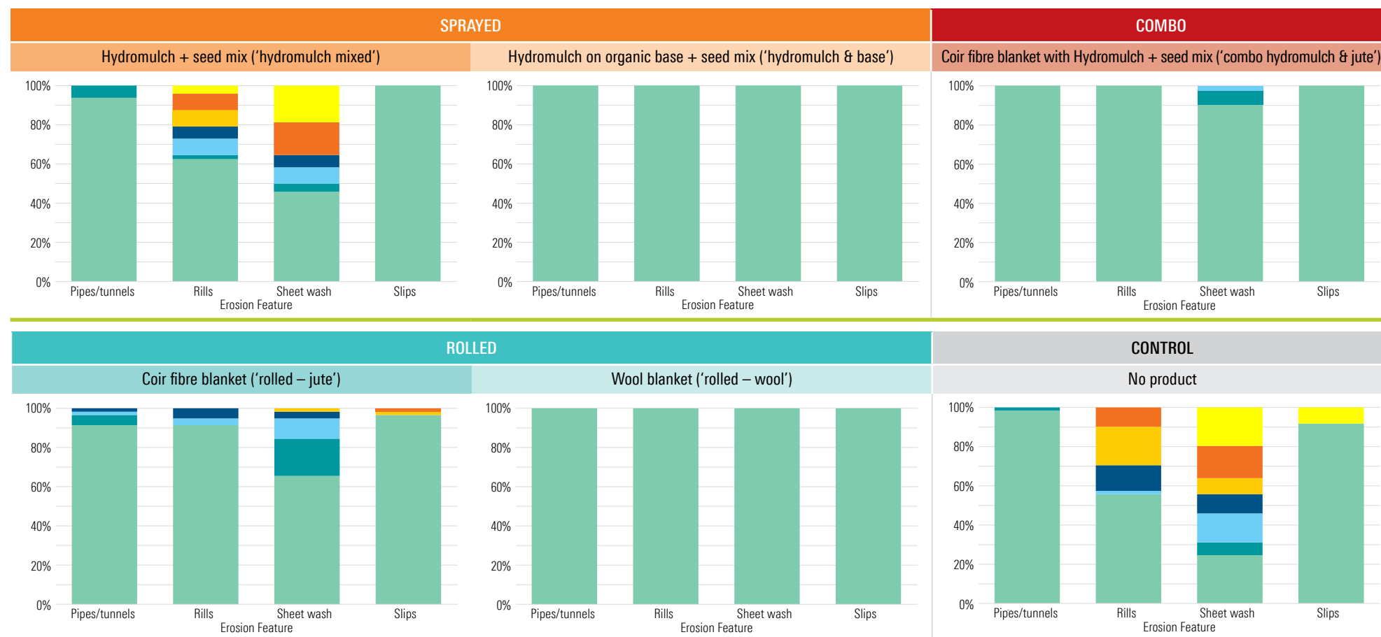
FIGURE 10: Graph showing the PROPORTION OF THE DIFFERENT TYPES OF EROSION FEATURES in grids across the five different treatments and control ('no product'), for grids that were classified as 'mainly loess subsoil'. Data for the % cover categories is based on the proportion of grids that were classified as one of six cover categories. Data is presented for the last round of monitoring only, undertaken approximately 30 months (2.5 years) after site setup.
