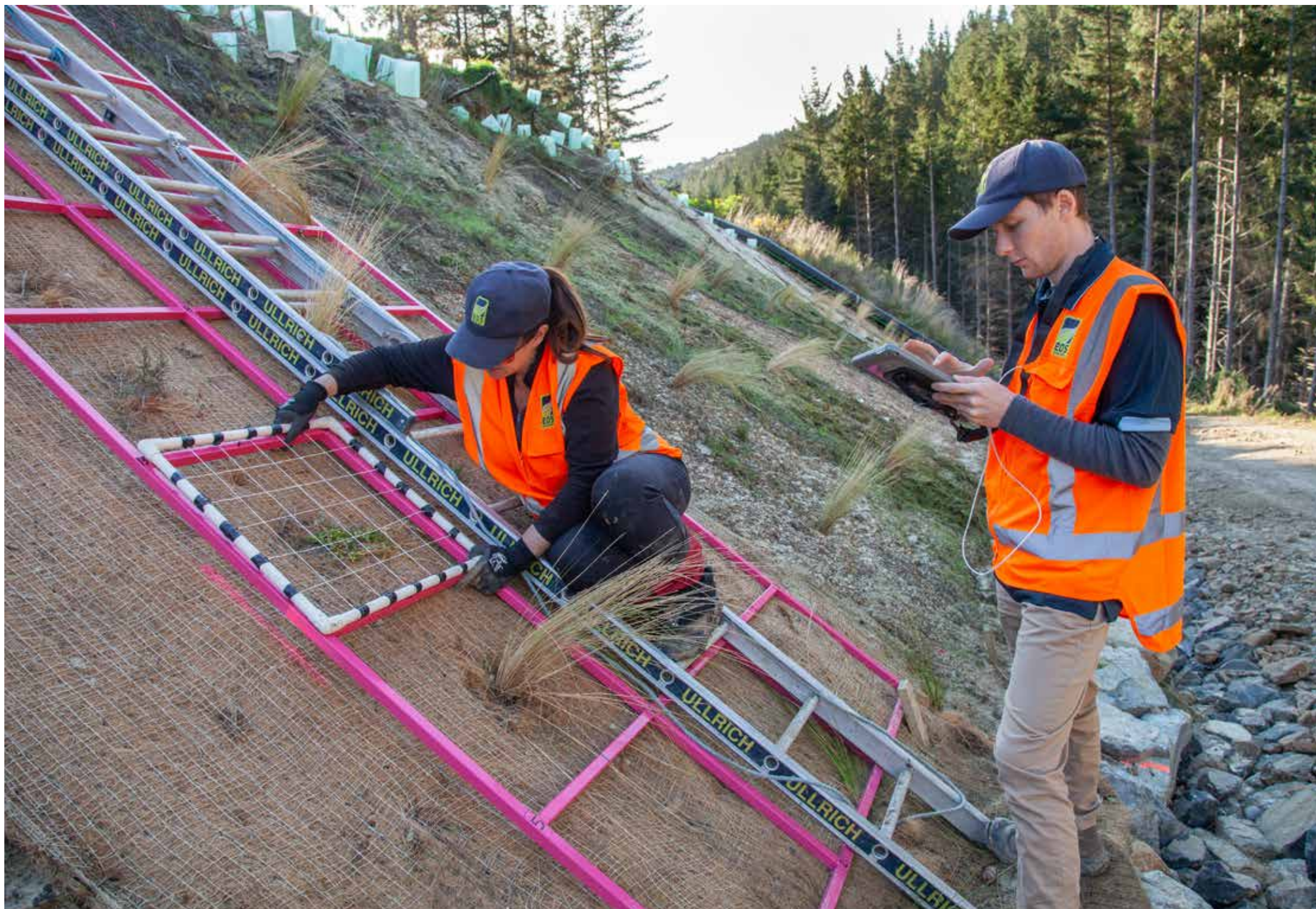
FIGURE 6: The science team using the monitoring grid and ladder to quantify conditions within 24 replicate grids for each plot in the cut face experiment.
